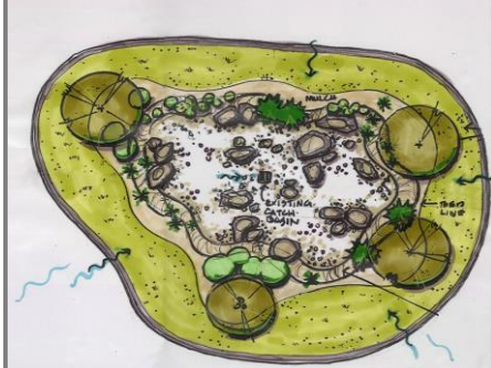
Bio-islands are landscaped drainage systems that filter and clean stormwater before it leaves the property. These designs can be incorporated into existing sites and make great projects for businesses and residents to demonstrate their dedication to water quality improvement.
