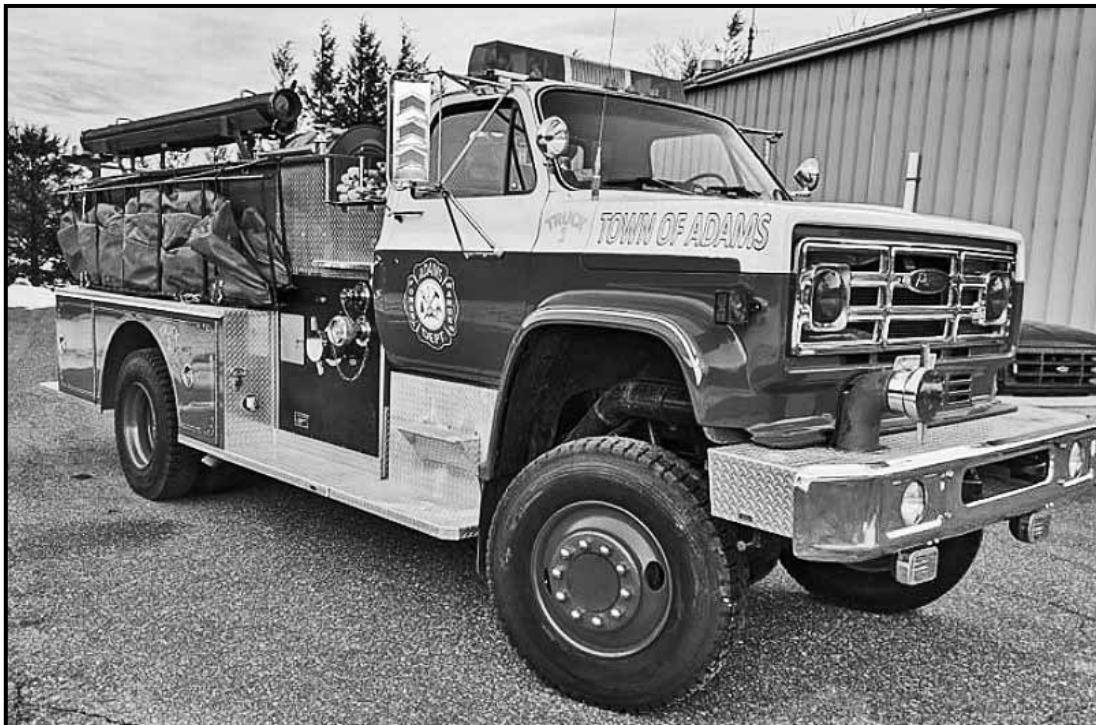
The Adams Forest Wardens' 1986 Pierce Pumper four wheel drive Fire Truck, equipped with a 1,000 gallon per minute pump and 500 gallon poly storage water tank.
